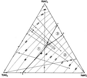
System point Composition Temp.  $X_{\text{NaNO3}}$  $X_{\text{TlNO}_3}$ °C (mole (mole fraction) fraction) (Tl, Na, Li)NO<sub>3</sub> 0.1530.569121.5 (Tl, Na, Rb)NO3 0.331 0.268 154.5
